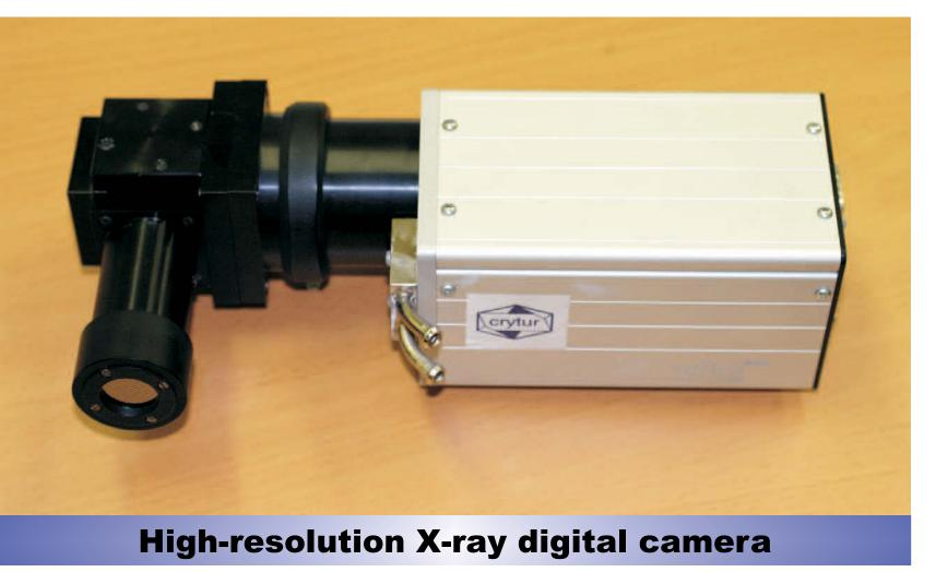
The high resolution imaging screen is the basic part of the high-resolution imaging system. The very thin imaging screens are based on the YAG:Ce or the LuAG:Ce single crystal scintillation material.
